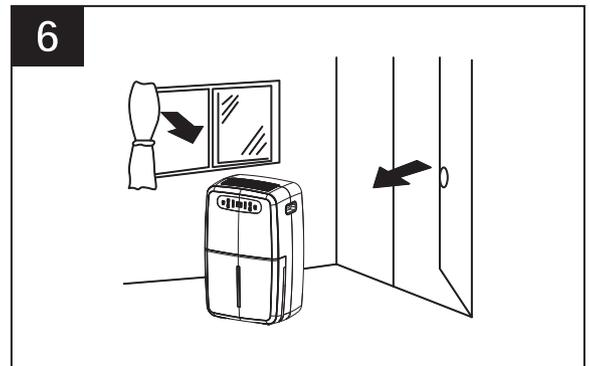
7. Keep the machine away from any type of heat source.
